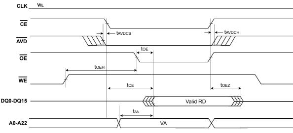
Figure 9: Asynchronous Mode Read
