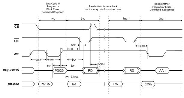
Figure 17: Read While Write Operation
