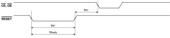
**Reset Timings NOT during Internal Routines**
