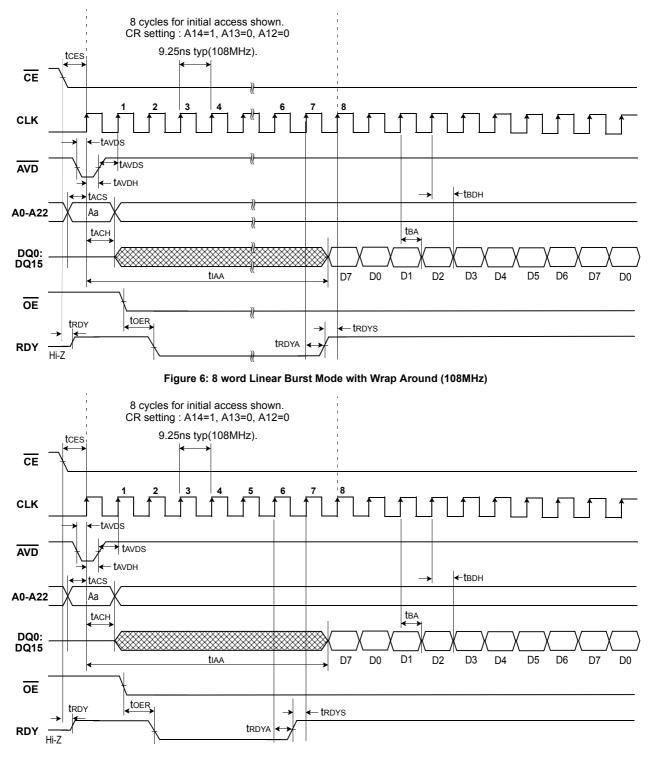
Figure 7: 8 word Linear Burst with RDY Set One Cycle Before Data
